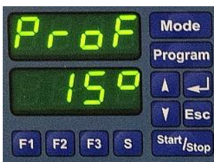
Oven control by setting air temperature as a temperature-time profile
