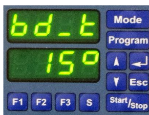
Oven control by setting desired object temperature as a temperature-time profile
